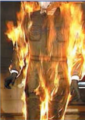
Non-Flame Resistant Clothing Non-flame resistant clothing ignites and continues to burn
